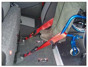
LA SICUREZZA E' GARANTITA TRAMITE UN SISTEMA DI ANCORAGGIO CARROZZINA A 4 PUNTI E CINTURA DI SICUREZZA A 3 PUNTI PER IL PASSEGGERO DISABILE.
